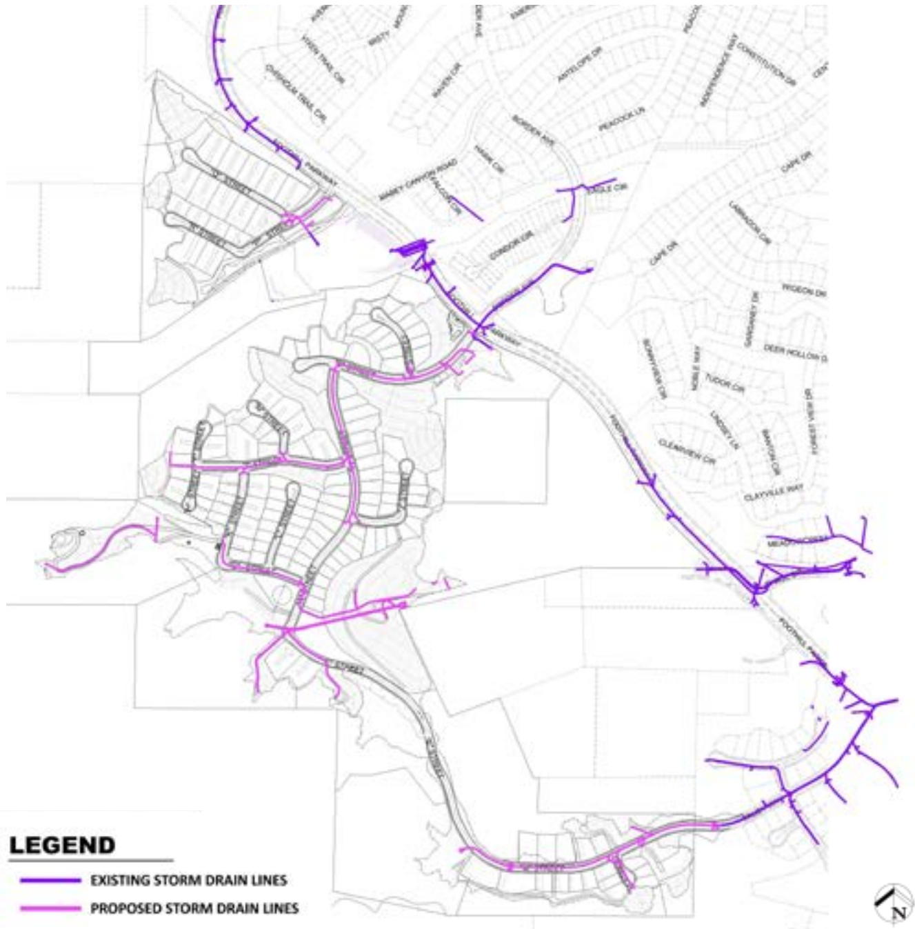
EXHIBIT 3-13 CONCEPTUAL STORM DRAIN PLAN
