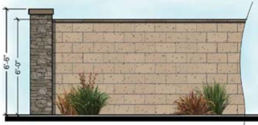
WALL: W-01 PILASTER: W-02. 6'-0" TALL SPLIT FACE BLOCK WALL W/ PRECAST CAP 6'-6" TALL STONE VENEER PILASTER W/ PRECAST CAP
